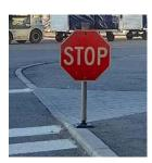
STOP signs and STOP lines are positioned to provide safe clearance for vehicle traffic and safe clearance for aircraft (wingtip & taxi clearance).
