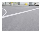
STOP Lines are a single solid white line and are used to indicate a MANDATORY STOP to the driver. A STOP sign is typically installed at a STOP line. All drivers are expected to STOP at a STOP line whether or not there is a STOP sign.
