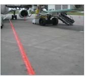
A single red line outlines the boundary of the bridge movement area. Parking is not allowed within the marked area where the bridge can travel unless the aircraft is parked on gate and the vehicle is being used to actively service that aircraft.
