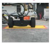
A yellow rectangle outlined in red indicates the area on the Apron where a bridge's wheels are parked when the bridge is not in use. Parking is not allowed in this area.
