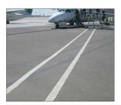
Pedestrian Crossings are indicated by two parallel white lines. Pedestrian Crossings indicate where people are allowed to walk on an Apron, such as when crossing breezeways or between the aircraft stand and the terminal building at a Ground Loading Operational Stand. Pedestrians in marked crossings (or walkways) have the right-of-way over vehicles.
