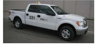
Company name and identification must be of sufficient size and contrast to be visible and readable from a minimum distance of 15 meters. (example: Large trucks (lift trucks/catering trucks) must have numbers a minimum of 30 cm (12 inches) high on both sides of the vehicle.
