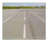
Vehicle Service Roads (VSRs) are indicated by two solid white lines at least 7.5 meters apart with a single broken center line. VSRs may be two-way traffic, or one-way traffic. (Ref. 6.7 for VSR right-of-way rules)
