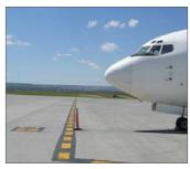
An Aircraft Parking Boundary Line is a single yellow broken line, often parallel to the Apron Taxiway and is used to outline aircraft parking pads. Aircraft are parked behind Aircraft Parking Boundary Lines to ensure they are safely separated and clear of taxiing aircraft.
