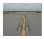
Enhanced Taxiway Center Lines are Taxiway Center Lines that are enhanced for 47.5 meters leading up to the Runway Holding Position Markings, by the addition of broken yellow lines on either side of the solid yellow center line.
