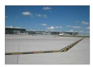
DA AVOP holders must not cross the Apron Limit Line (MAD Marking) to exit an Apron onto a Taxiway unless under escort by a D AVOP holder. D-Tow operators must never cross the Apron Limit Line (MAD Marking) with the tow vehicle or any part of an aircraft without permission from Air Traffic Control (ATC).
