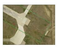
The protected area of a surface designated for the landing and take-off of aircraft. This protected area runs between the extended runway Hold Lines on each side and inside the localizer antenna arrays on each end of the runway. ATC must ensure this area is clear before clearing an aircraft to land or take-off on that runway.
